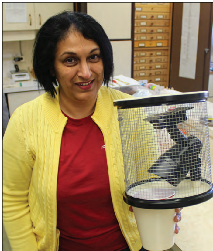
Dr. Christine Noronha of Agriculture and Agri-Food Canada in Charlottetown, PEI with a 3D printed prototype of her newly designed "Noronha Elaterid Light Trap" (NELT).
